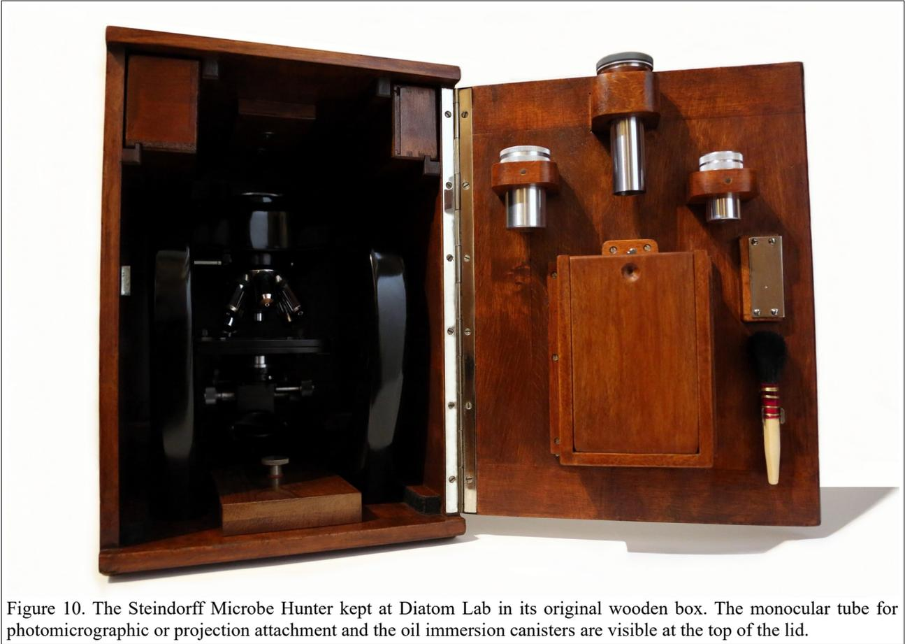
Figure 10. The Steindorff Microbe Hunter kept at Diatom Lab in its original wooden box. The monocular tube for photomicrographic or projection attachment and the oil immersion canisters are visible at the top of the lid.
